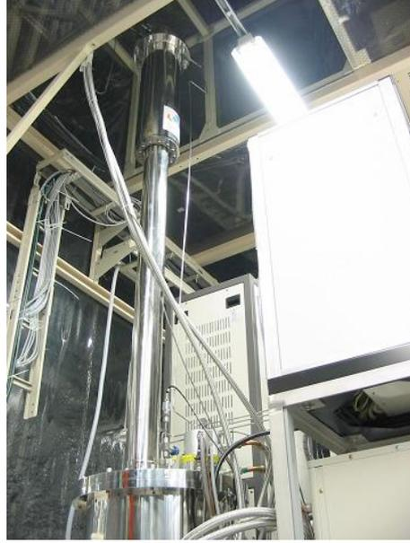
**FIGURE 1.** The distillation system in Kamioka Observatory. The height of the distillation tower is about 3m.
