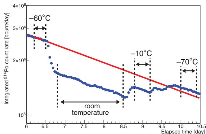
**Fig. 4.** An example of the variation of the integrated count rate of  $^{214}\text{Po}$  in the 80 L radon detector with different dew point values. The solid red line shows a fit to the data at  $-60^\circ\text{C}$  with the expected radon decay constant. The vertical dashed lines indicate the regions used to obtain the CF.
