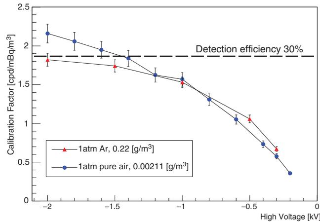
**Fig. 3.** The calibration factor of 80 L radon detectors as a function of supplied high-voltage value. The Ar and air data were taken with the calibration systems in Kobe and in Kamioka, respectively. The error bar shows systematic uncertainties of the measurements. Here, the uncertainties of the dew point measurement and the radon concentration are included. See text for details on the dashed line.
