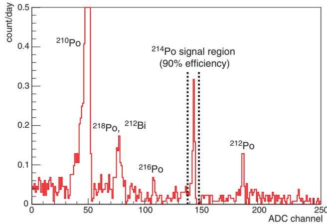
**Fig. 6.** Pulse height spectrum in the background run with purified air under 1 atmospheric pressure and  $-2.0$  kV high-voltage value in Kobe. ADC channel 137–147 was used as the  $^{214}\text{Po}$  signal region. The huge peak at around 50 ADC count is due to  $^{210}\text{Po}$ , which was accumulated during the calibration measurements.
