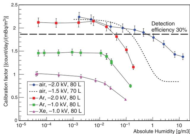
**Fig. 5.** The calibration factor of the 80 L radon detector as a function of absolute humidity. The dotted line shows that of the 70 L radon detector [4]. The air data were taken in Kamioka, and others were taken in Kobe. For details on the dashed line and the error bars, see Fig. 3.
