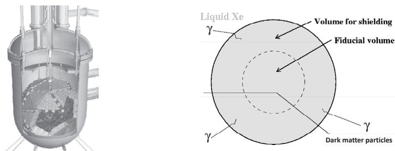
Figure 2. Structure of the 800-kg detector (left). Liquid xenon fills the central part and is surrounded by 642 photomultiplier tubes. Since the dominant background is caused by gamma rays from the PMTs, which can be absorbed by the exterior layer of the liquid xenon, a low-background experiment would be possible if the inner radioactivity was shown to be low (right).
