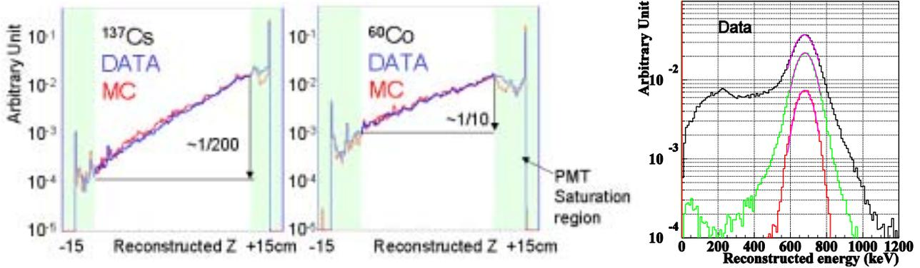
Fig.3 (left) The vertex distribution for Z position in source run. +15cm shows the wall near the source. (right) The energy distribution of Cs source run in each fiducial volume. From the outside to inside, all volume, 20cm fiducial, and 10cm fiducial volume are shown respectively.
