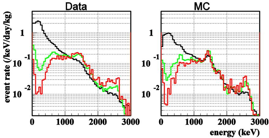
Fig.4 The spectrum of background run in each fiducial volume. From the upper to lower in low energy region shows, all volume, 20cm fiducial, and 10cm fiducial volume are shown respectively.
