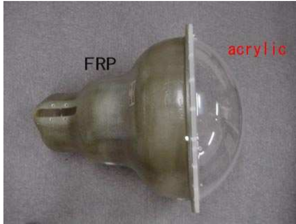
Figure 2.10: PMT case used in SK-II and SK-III
