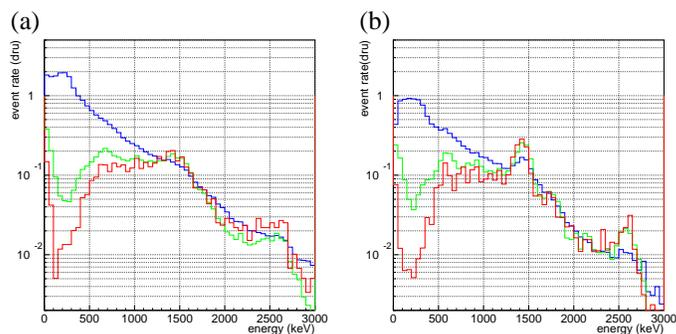
Figure 4. Energy spectrum of normal run: (a) Data and (b) MC. The blue, green, and red lines correspond to full volume, 20cm fiducial volume, and 10cm fiducial volume, respectively. The event rate increase at the lowest energy region of red and green lines are due to the detector wall effects (see text).
