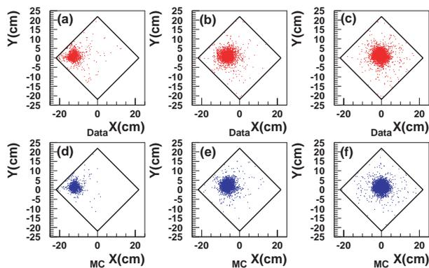
Figure 2. Vertex reconstruction performance: (a),(b),(c) Data and (d),(e),(f) MC. The reconstructed vertex positions of collimated gamma source runs are plotted. (a),(c) Hole-C (left side), (b),(e) Hole-B (left-center), and (c),(f) Hole-A (center) are used.
