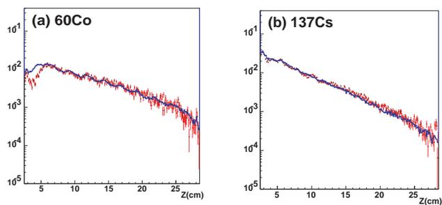
Figure 3. Self shielding performance: (a)  $^{60}\text{Co}$  and (b)  $^{137}\text{Cs}$ . The blue line and red plots correspond to MC and Data, respectively. The collimated gamma rays are injected horizontally from Hole-A (center) at  $Z=0(\text{cm})$  position. The reconstructed vertex positions are plotted. The wiggles are due to grid effects of the current reconstruction tool and will be improved.
