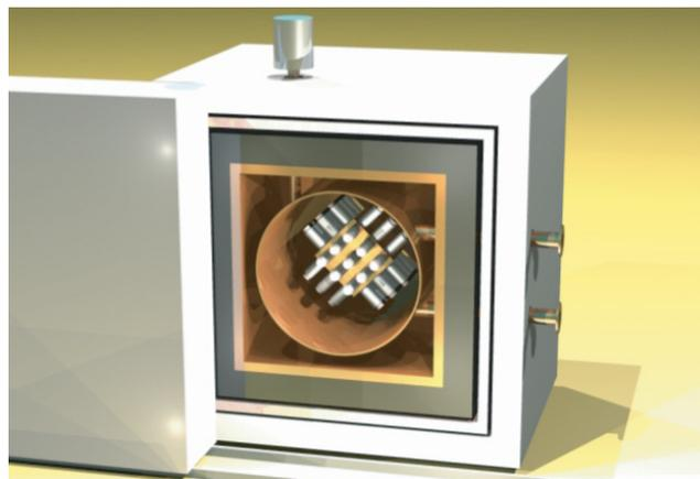
Figure 1. XMASS prototype detector. 100kg liquid xenon and 54 low-background PMTs are used. PMTs are attached to the 30L OFC chamber through 5mm thickness  $\text{MgF}_2$  windows. They are put into a heavy shield in a clean room. The XMASS prototype detector is located in Kamioka Observatory, ICRR, Univ of Tokyo, in Kamioka mine.
