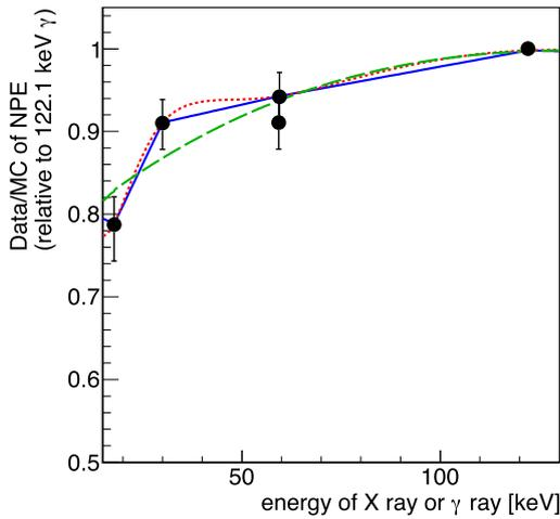
**Fig. 3.** MC correction for the NPE non-linearity. The value at 122.1 keV  $\gamma$ -ray is normalized to 1. The black dots show the results from different calibration sources. Examples for the  $f_{model}$  functions are shown as the solid (linear interpolation), the dotted (spline interpolation), and the dashed (6-th degree polynomial fitting) lines.
