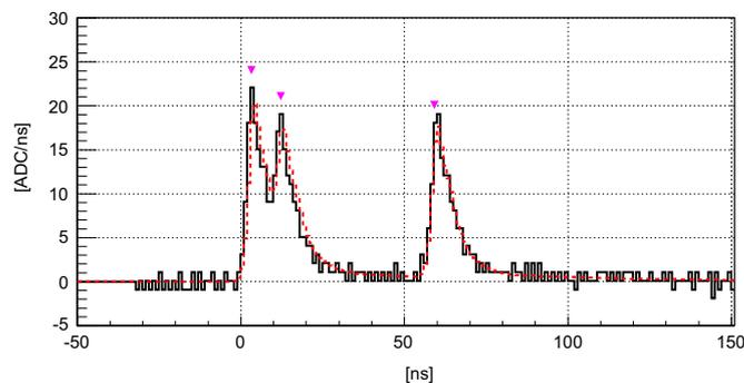
**Fig. 1.** A typical raw waveform in a PMT (solid line) overlaid with the reconstructed waveform as the sum of 1 PE pulses (dashed curve) for the 122 keV gamma-ray from the  $^{57}\text{Co}$  source placed at  $Z=0$  cm. The triangle markers indicate timings of the decoupled 1 PE pulses.
