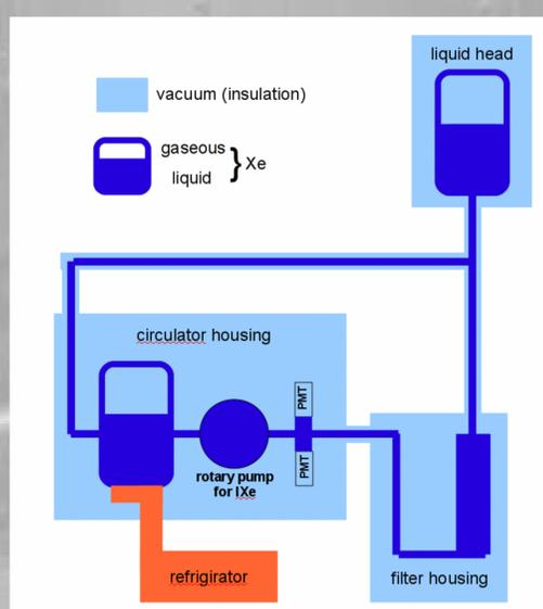
**Figure 1:** Schematic overview of IXe circulation system
