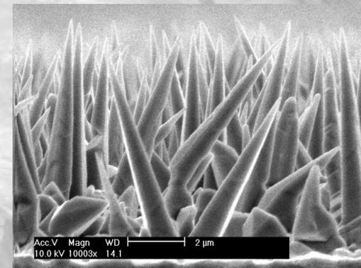
**Figure 2:** Copper micro-tips grown at SNU in Korea (reproduced with permission)
