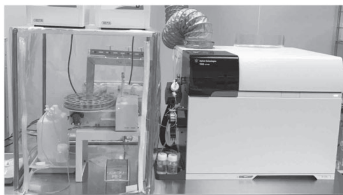
Fig. 1. Picture of the ICP-MS “Agilent7900” in the Kamioka clean room. The auto-sampler is fully covered by the class 100 clean booth to reduce contamination from the outside.
