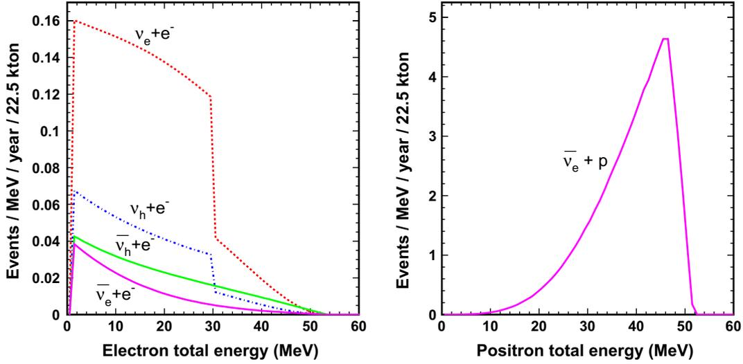
**Fig. 2.** Expected energy spectra of elastic scattering recoil electron (left) and inverse beta decay positron (right) in SK assuming neutrino flux of  $3.0 \times 10^2 \text{ cm}^{-2} \text{ s}^{-1}$  without energy resolution included. The discontinuity of some spectra at 29.79 MeV is caused by the spikes shown in the expected neutrino energy spectra in Fig. 1.  $h$  represents  $\mu$  and  $\tau$  components.
