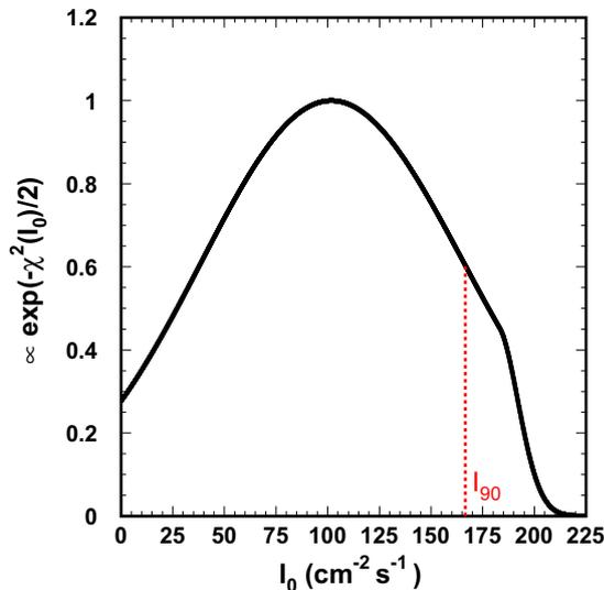
**Fig. 5.** Likelihood function as a function of monopole-induced neutrino flux ( $I_0$ ), which is defined as proportional to  $\exp(-\chi^2(I_0)/2)$ . The dashed line represents the 90% C.L. limit on  $I_0$ . The deviation from the Gaussian shape beyond  $I_0 = 183.4 \text{ cm}^{-2} \text{ s}^{-1}$  is due to the restriction of  $\alpha \geq 0$ .
