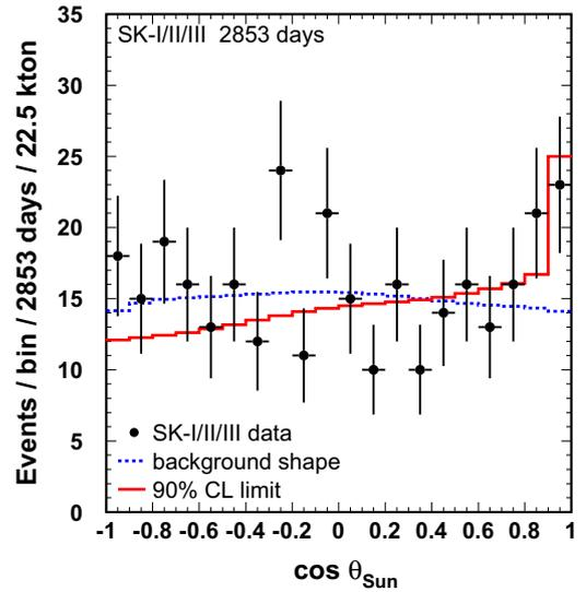
**Fig. 3.** Angular distributions with respect to the expected neutrino direction from the Sun. The points with error bars show the data events. The solid histogram represents the fitting result when the monopole-induced neutrino flux is equated with the 90% C.L. upper limit obtained in this analysis, and the dashed one the result when only background is used for the fitting.
